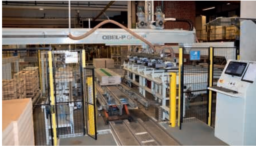
The new packaging line for Huntonit is now running 24/7 and packs up to 72 workpieces per minute.
