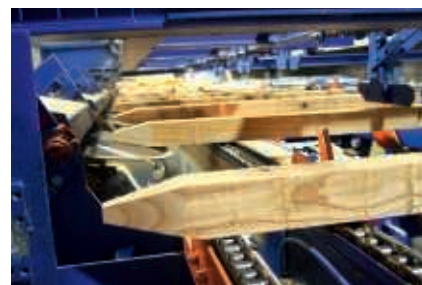
The post-pointing unit in a line similar to the BSW installation
